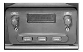
**VOL** (**Volume**): Turn the knob to increase and to decrease volume. The left VOL knob controls the left headphone and the right VOL knob controls the right headphone.
